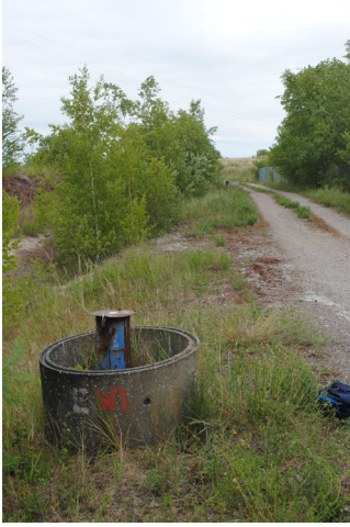
CMS monitoring well on footpath entrance to site
